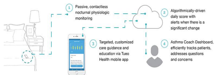
Figure 1 - Asthmapolis Sensor Functionality
