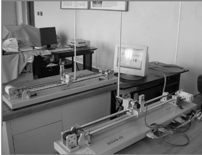
Figure 1: Dual Inverted Pendulums used for Synchronization Experiment [Dongfang Zhu & Di Zhou, 2008]
