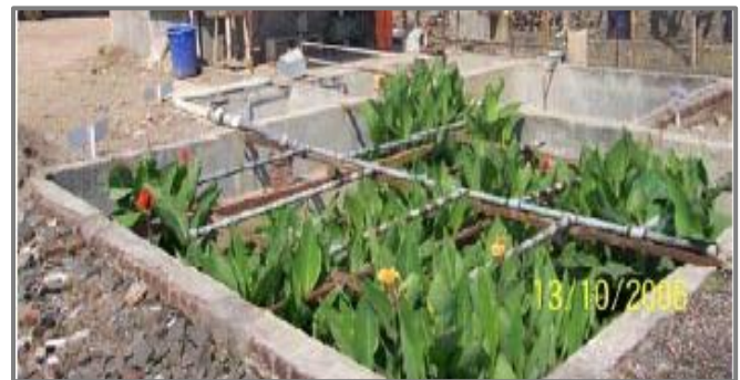
Figure 6: An Example of Pilot Model System of Aquatic Plants Phytoremediation Process done by Sayali Joshi from Shrishti Eco-Research Institute [Sengupta et al., 2008]
